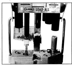
**STATION 5** Immediately move the shell into the shell holder at STATION 5 and complete the crimp. You should have a perfectly crimped shell with a nice, tapered end.
