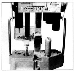
**STATION 4** Place the shell under the proper crimp starter. Keep an inward fold of the shell mouth toward The front for proper alignment with the segmented starter. Depress the handle to a full stop. Some shells may require a two-second pause to set the plastic.
